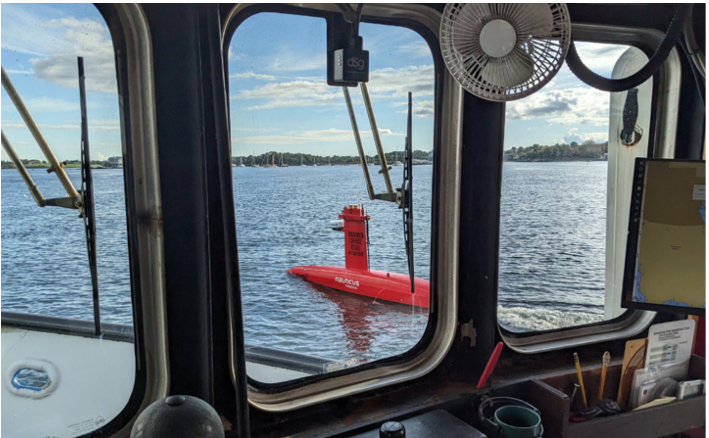
A DriX uncrewed surface vehicle as it transited to a survey site as seen from the NOAA R/V Gloria Michelle .
